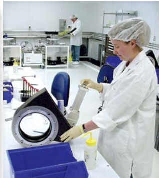
Valve assembly in Class 1000 Clean Room
