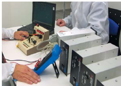
Calibration of Intellisys adaptive pressure controllers
