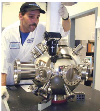
Manual CMM (coordinate measurement machine) inspection
