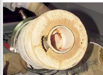
Water-cooled / particle trap for CVD
