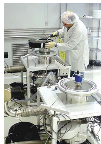
Leak testing pendulum valves
