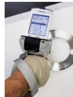
XRF inspections provide precise chemical makeup of materials
