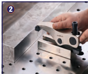
Upper casing is slid to slide, it is brought to position on work pieces.
