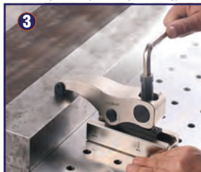
Fix upper bolt of lug to work piece.
