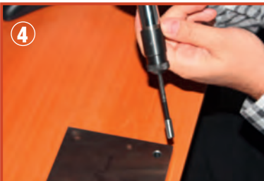
Extracted pin is removed from adaptor.
