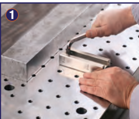
Bottom slide is made suitable to work piece and fixed.
