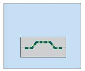
The resin continues to disperse as the mold closes, and the entire cavity is filled after complete closure.
