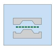
The impregnated fiber mats are placed into the mold. The time factor is relevant here because the reaction has already started. This is why robots are often used to perform this step.
