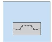
The binding powder added during stacking melts due to the heat impact and fixes the mats or fabrics in the correct shape.
