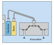
The cavity is evacuated after the mold is closed. This prevents air inclusions in the final product.
