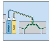
The resin/hardener mixture is injected into the cavity at a defined pressure, while the preform is impregnated with resin. Curing of the resin starts once the cavity is filled.
