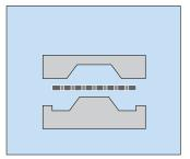
The package is molded into the required shape using a dedicated mold.
