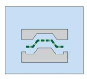
After curing, the mold is opened and the part can be demolded.
