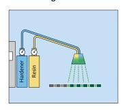
Dry fiber mats or fabrics are impregnated with the resin/hardener mixture.
