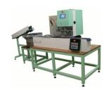
1 colour pad printing system for marking on closures in colour. Loading autmatically, pre-treatment, pad printing and autmatically reject
