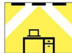
Direct light and walls illumination
