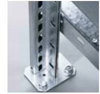
Floor fastening for shelves with a height/depth ratio of \geq 5:1 . This type of shelving must be secured against tipping (wall or foot fastening).
