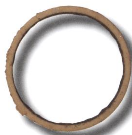
Cooling water pipes after less than one year's operation with Tekleen filtration.
