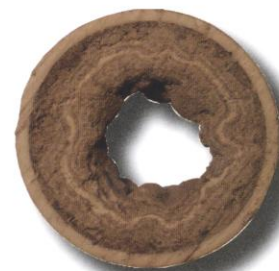
Cooling water pipes after less than one year's operation without filtration.
