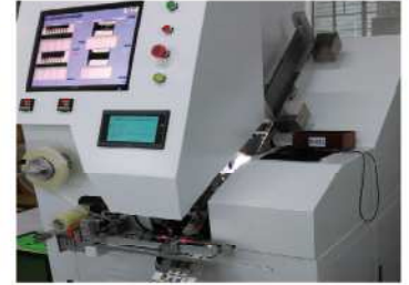
3 in 1 Auto inspection machine (Flatness/ Visual/ Taping)
