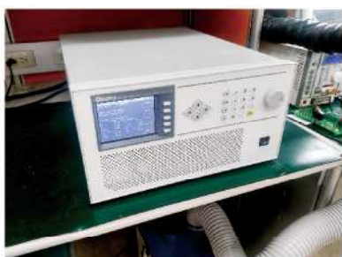
Programmable AC Source Model (VAC 300volt)
