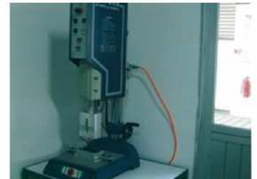
Ultrasonic Welding for Sealing Plastic Case
