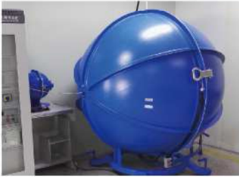
Integrating Sphere (for Testing LED Luminous)
