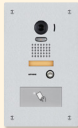
JP-DVF-HID* Card Access Video Door Station • HID® ProxPoint® Plus Proximity Card Reader • PTZ camera • Stainless steel panel • Weather and vandal resistant • Flush mount (back box included)
