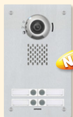
IX-DVF-4 IP Addressable Video Door Station • 4 call buttons • PoE or 24V DC • SIP compatible • Fixed camera • Stainless steel panel • Weather resistant • Flush mount (back box included)
