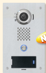
IX-DVF-P* IP Addressable Card Access Video Door Station • HID® multiCLASS SE® Proximity Card Reader • PoE or 24V DC • SIP compatible • Fixed camera • Stainless steel panel • Weather and vandal resistant • Flush mount (back box included)
