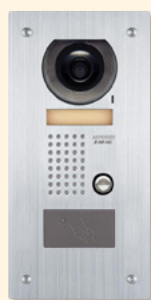
JF-DVF-HID* Card Access Video Door Station • HID® ProxPoint® Plus Proximity Card Reader • Fixed camera • Stainless steel panel • Weather and vandal resistant • Flush mount (back box included)
