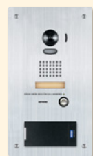
IS-IPDV † IP Addressable Video Door Station • PoE capable • PTZ camera • Aluminum die cast cover • Weather and vandal resistant • Surface mount → p. 78
