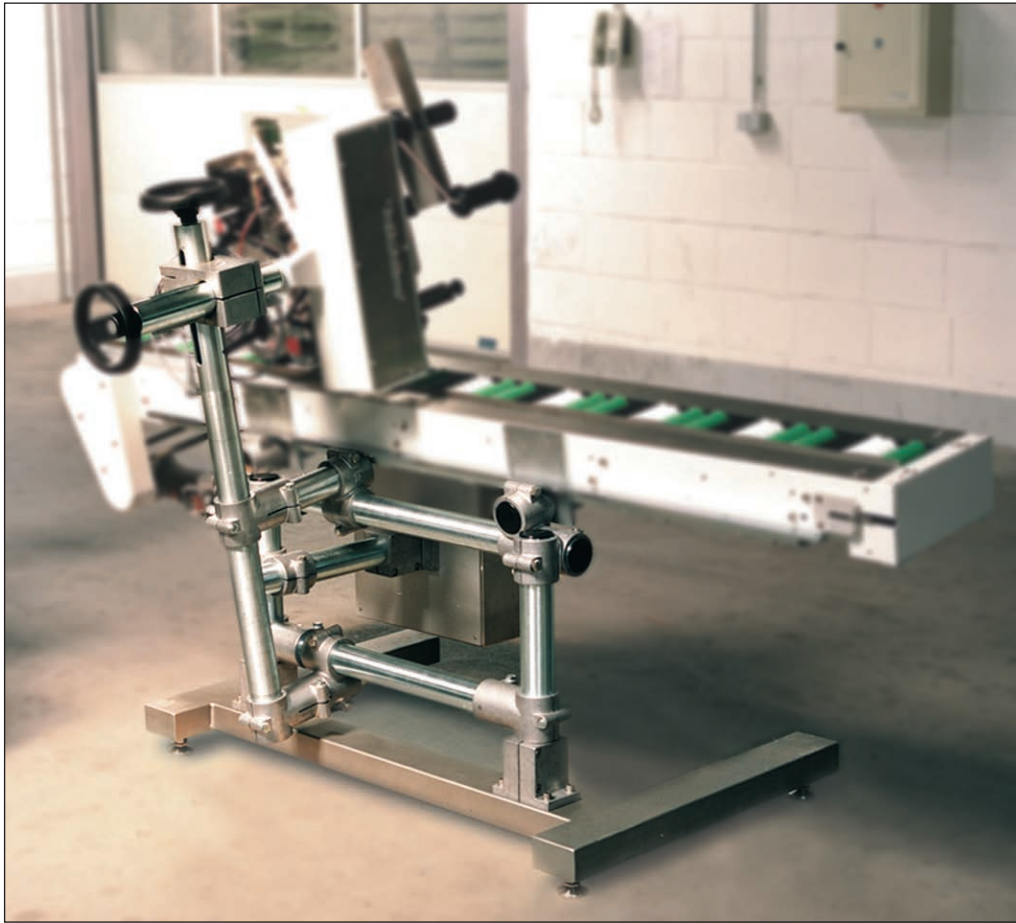
Frame for a labelling machine.
