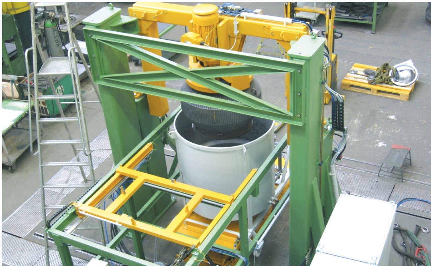
ESD application with igus® E2/000 e-chains® in a centrifuge for de-oiling, drying, rinsing, coating and rust protection
