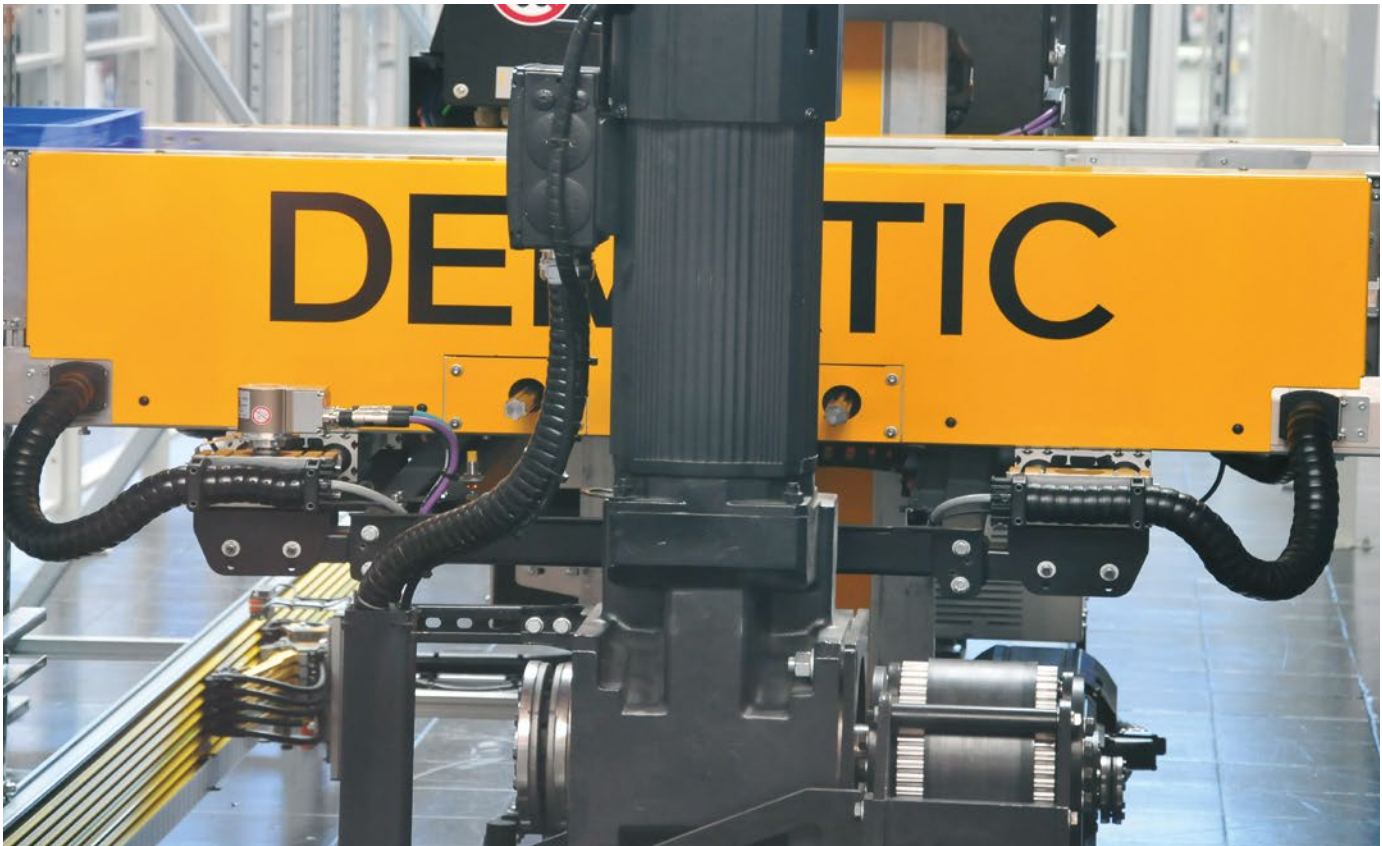
triflex® R in storage and retrieval system
