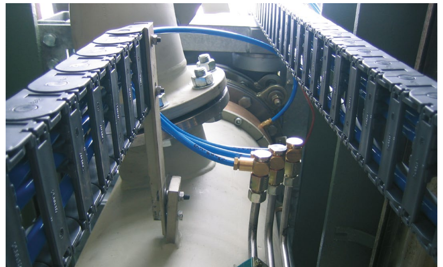
igus® ESD version of the E2/000 system in a tank filling station
