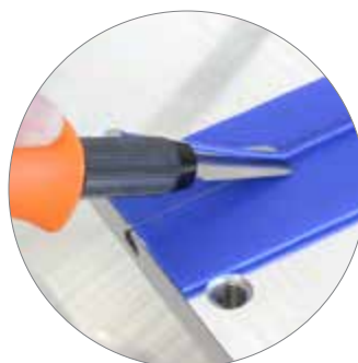
Easy removal of the welding bead with the supplied tool
