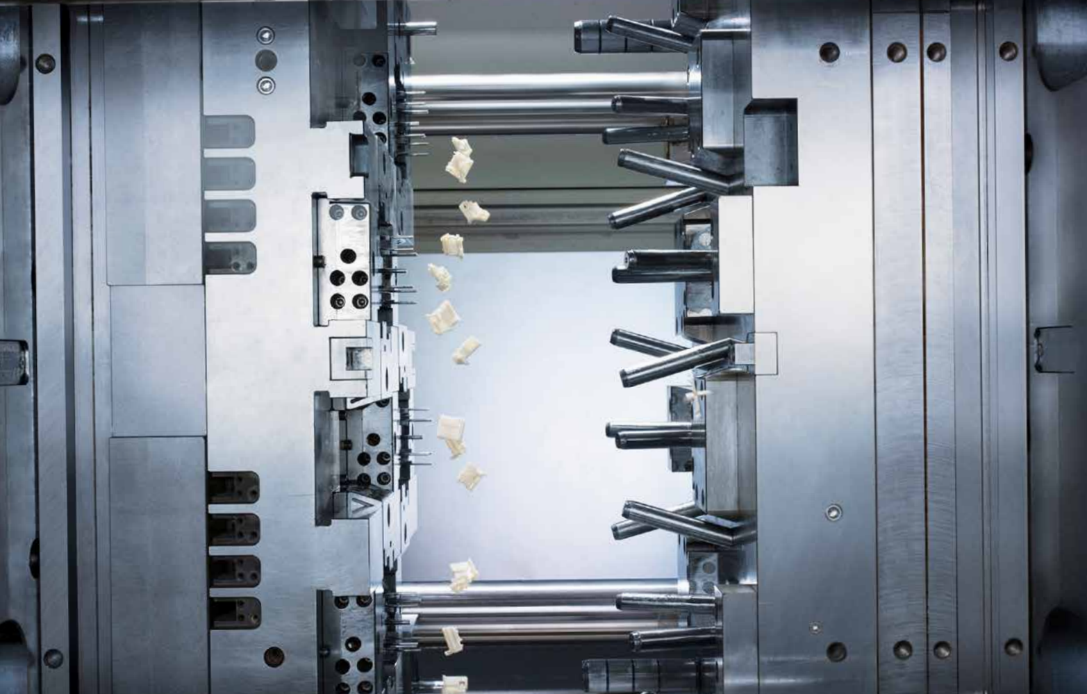
Cavity pressure monitoring during injection molding reduces the costs of quality assurance.
